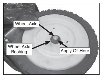
Figure 10. Wheel axle lubrication.
